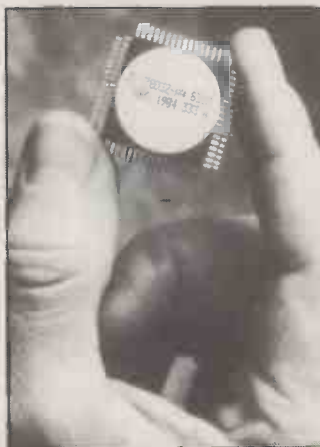
The Microvax II is built around DEC's own 78032 chip and approaches the power of the Vax II/780 mini.
